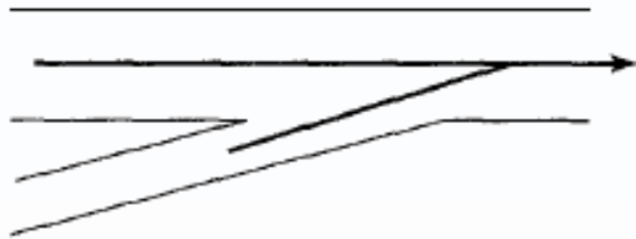
(b) Merging movements join to form a single traffic stream.
