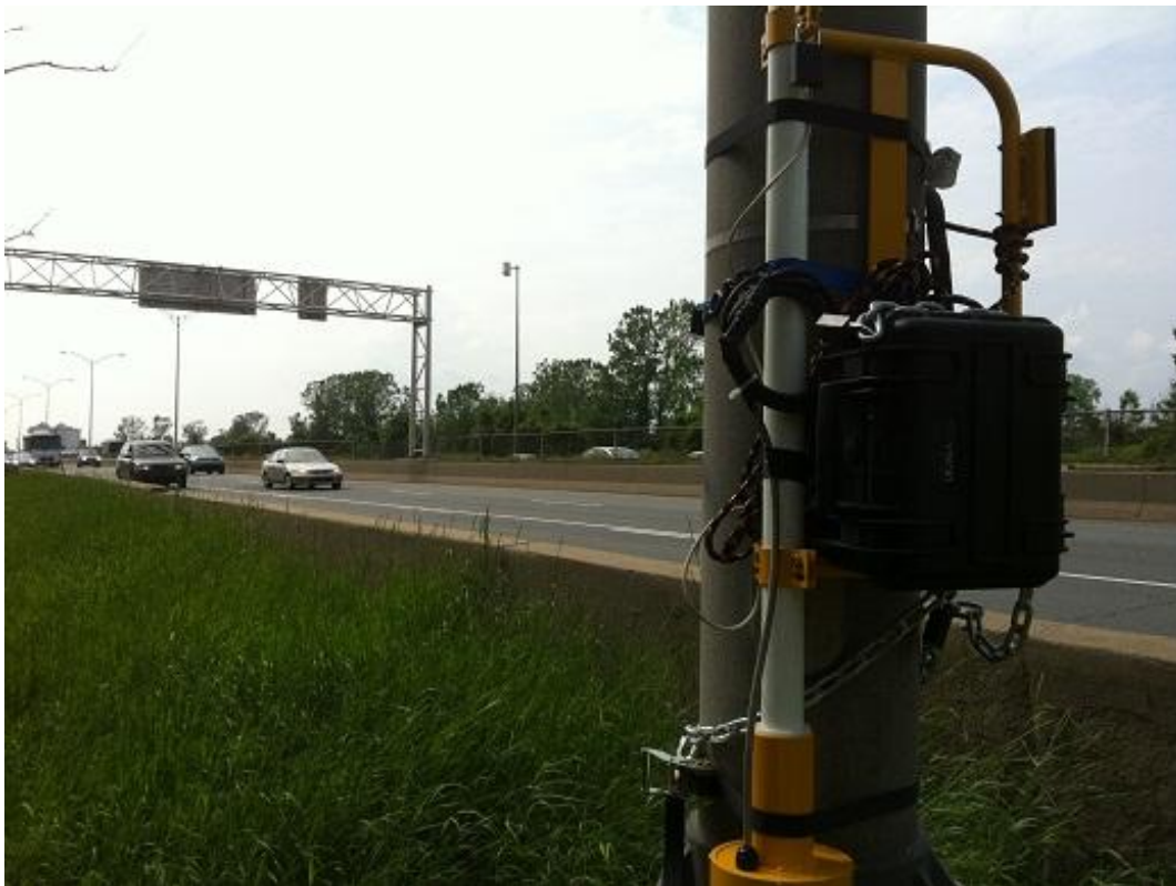
Figure 20 – Base of pole installation for MTG-Cam20-E-55e-Sortie.
