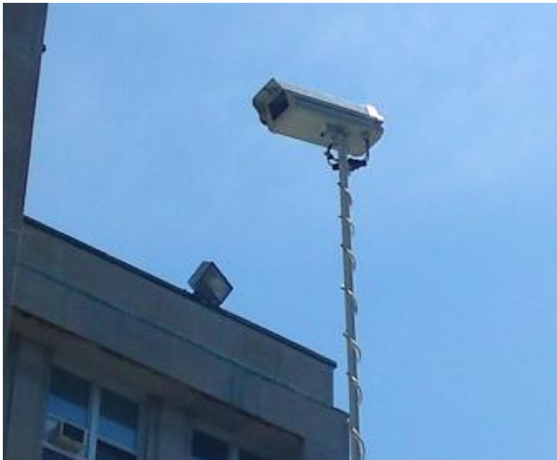
Figure 19 – Free-standing camera housing deployed to a height of 8 metres.
